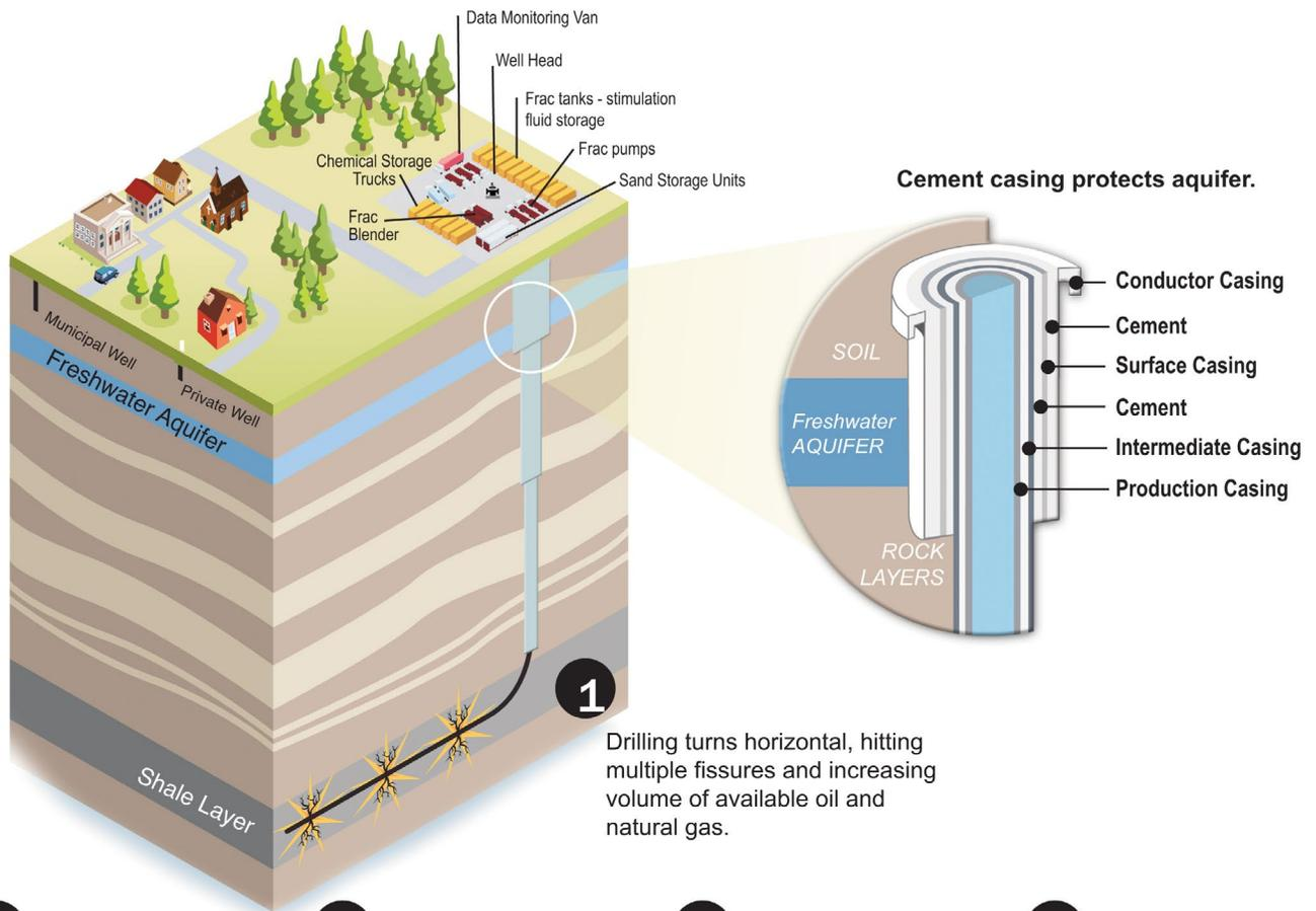
1 Drilling turns horizontal, hitting multiple fissures and increasing volume of available oil and natural gas.
