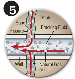
5 The fluid generates numerous small fissures in the shale, freeing trapped oil and gas that flow back up the pipeline to the wellhead. The sand keeps the fissures open to increase the flow of oil and natural gas.
