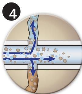
4 After drilling, the well is hydraulically fractured. A mixture of water, sand, and chemicals (fracking fluid) is pumped into the well at high pressure.
