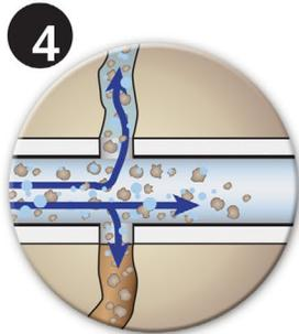
4 After drilling, the well is hydraulically fractured. A mixture of water, sand, and chemicals (fracking fluid) is pumped into the well at high pressure.
